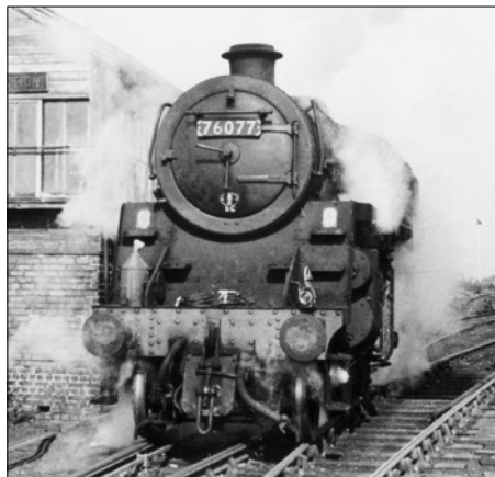
One of the five 2-6-0 BR Standard Class 4s based at 8G Sutton Oak, regularly used on the Earlestown Wagon Works test train.
