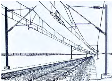
Typical Cantilever structure
