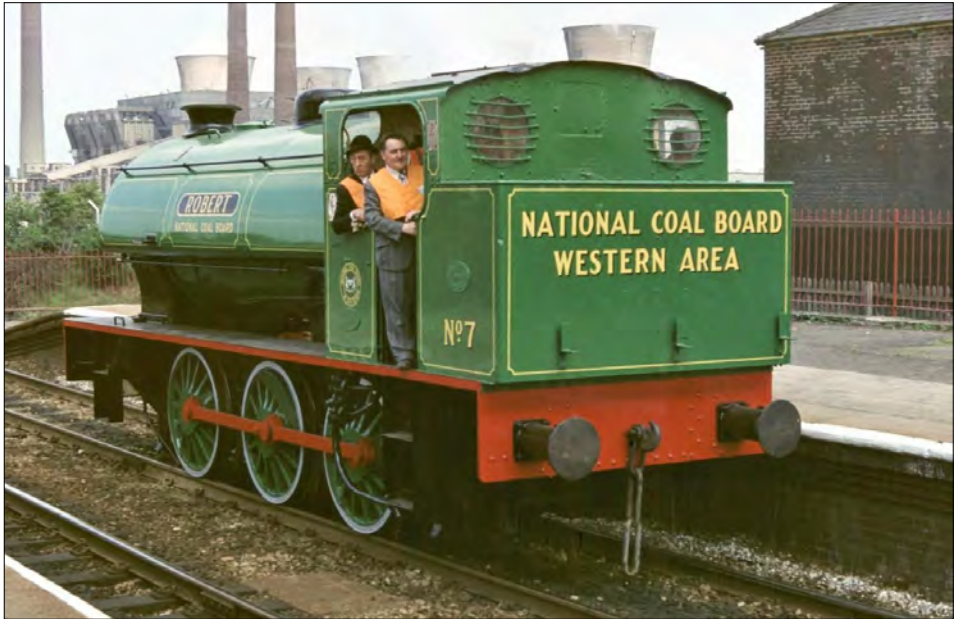
Above : National Coal Board Western Area No 7 Robert, a Hudswell Clarke 0-6-0ST built in 1943 which arrived at Bold Colliery in 1978, passes through St Helens Junction en route to taking part in the Rainhill 150 Celebrations in 1979. This locomotive is preserved on the Great Central Railway. Photo : Rod Dixon Collection
