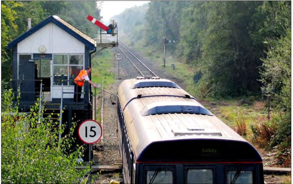
Above : Rainford Junction (c.2006) - the signalman hands the token via a pole to the driver of a Kirkby bound Class 142 unit approaching the down main starting signal. Below : Several years later (c.2016) after the signalbox had been refurbished, the driver of Manchester Victoria bound 150.228 brings his train to a stand to hand over the token to the signalman, before proceeding into the station.
