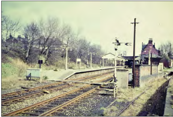
Above : Garston Station in 1970. The signal is Cressington's Down Distant, which was moved to the top of the post when Garston Signalbox closed and the Section signal was taken away.
