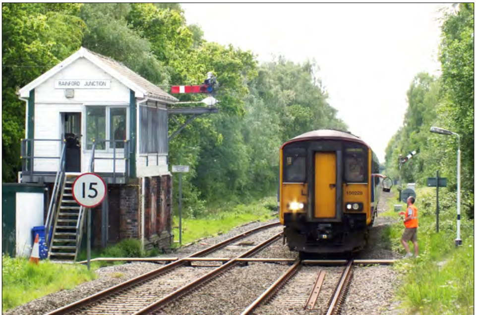
Above : Rainford Junction (c.2006) - the signalman hands the token via a pole to the driver of a Kirkby bound Class 142 unit approaching the down main starting signal. Below : Several years later (c.2016) after the signalbox had been refurbished, the driver of Manchester Victoria bound 150.228 brings his train to a stand to hand over the token to the signalman, before proceeding into the station.
