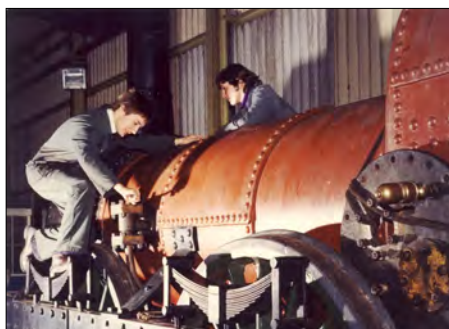
Above : Apprentices at Vulcan (Ruston Diesels) get to grips with 'Lion'. The 1838 locomotive was restored to full working order at the Newton le Willows works in preparation for its appearance at the Rainhill 150 celebrations.
