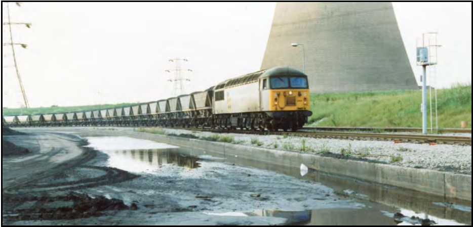
A class 56 locomotive heads towards the unloading plant at Fiddlers Ferry on 11 June 1992. The train is typical of Merry-go-Round services in the period from the late 1960s to the late 20 th century although the class 56 locomotives are a product of the 1970s. Photo by John Wilson
