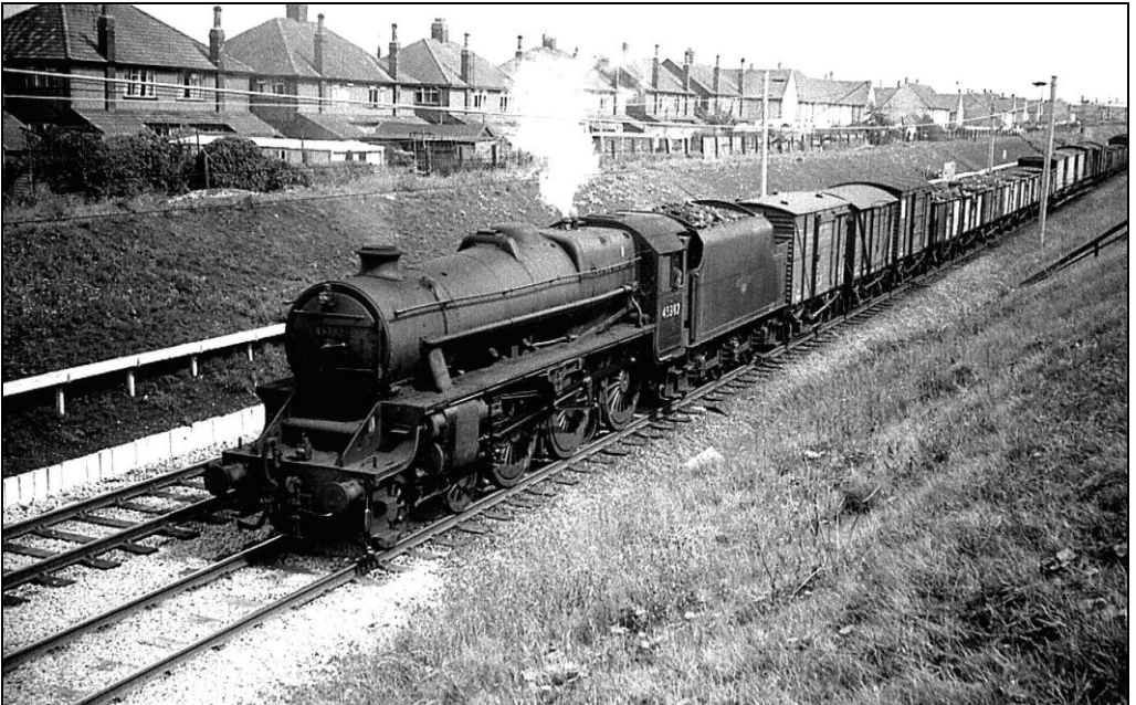
A goods train heads north through Runcorn in early 1960s. Although the wires were up by this time steam haulage was still a common sight. At the head of the train is a 4-6-0 5MT 'Black 5' locomotive of the type that Barry Nolan would have fired during the Liverpool to Stoke run of 1958. Photo by Roy Gough
