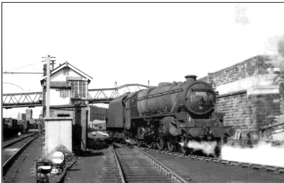
On the journey into Liverpool a glimpse was had of the extensive railway facilities at Brunswick. A Stanier 5MT 'Black 5' locomotive number 44777 is seen there in the early 1960s. Photo by Graham Earle
