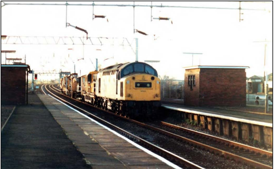
On 30 October 1986 locomotive number 97 405 'Ancient Mariner' is seen heading east through Ditton working a southbound engineers train. The engine started life as an English Electric Type 4 number D260. It became 40 060 in February 1974. The nose end of the loco was rebuilt, following an accident, with a central headcode, replacing the discs that the loco was originally fitted with. Photo by Terry Callaghan
