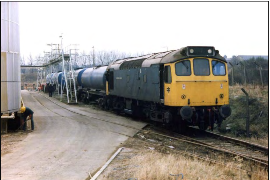
A view from inside the Hays works on 20 February 1986. A class 25 locomotive is seen shunting bogie tanks. Photo by John Wilson
