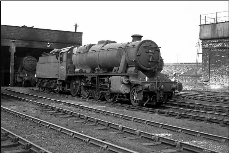
Widnes Locomotive shed on 20 September 1963. Ex LMS 2-8-0 8F locomotive number 48045 with a Fowler tender awaits its next duty. Photo by Brian Swinn
