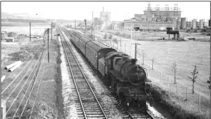
In 1964 Ivatt Mogul 2-6-0 locomotive number 43033 heads north along the former GCR/MR Widnes Branch towards Widnes East junction with a Liverpool Central – Manchester Central stopping service. The view was taken looking south from the Dans Road bridge. To the left can be seen works in connection with the construction of Fiddlers Ferry Power Station. Photo by Gordon Howarth
