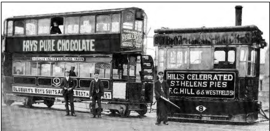
A St Helens steam hauled tram seen in 1895. Motive power is in the form of tramway engine number 8.
