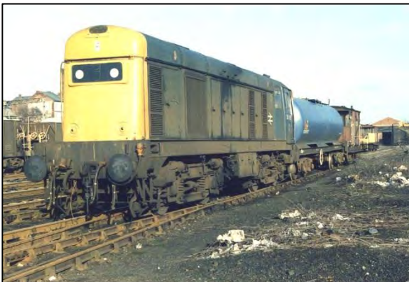
A class 20 diesel electric locomotive is seen at St Helens on 3 December 1985. The engine has behind it a bogie tank wagon of the type that used to work to Hayes chemical works. Behind the wagon is a standard BR brake van. Photo by John Wilson
