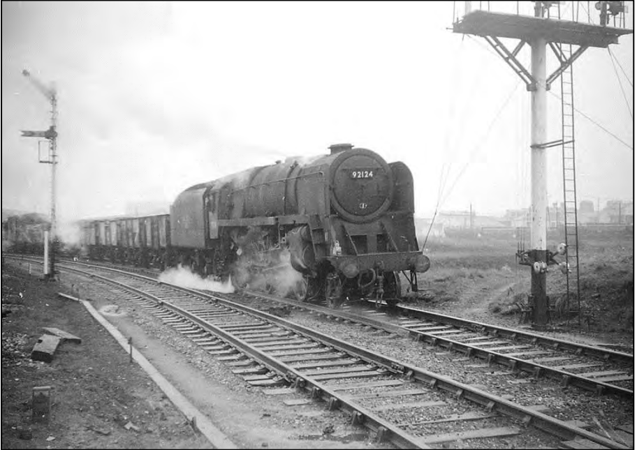
A BR 2-10-0 class 9F is seen on the approach to St Helens Shaw Street in the mid-1960s working a coal train from the Widnes direction. Duties such as this would have been commonplace for the firemen of depots such as Widnes and Sutton oak. Barry and his colleagues at Widnes did not normally have such a powerful locomotive at the head of one of their trains. Photo by Richard Mercer
