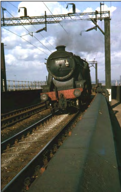
Left – An ex-LMS 2-8-0 8F locomotive number 48493 seen on the Widnes side of the Ethelfleda railway bridge in 1967. This is the type of locomotive that Dave Littler was on for 22 hours during Saturday 24 and Sunday 25 September 1960. One of the overhead gantries that had proved so difficult to erect is seen above the locomotive. Photo by Les Fifoot
