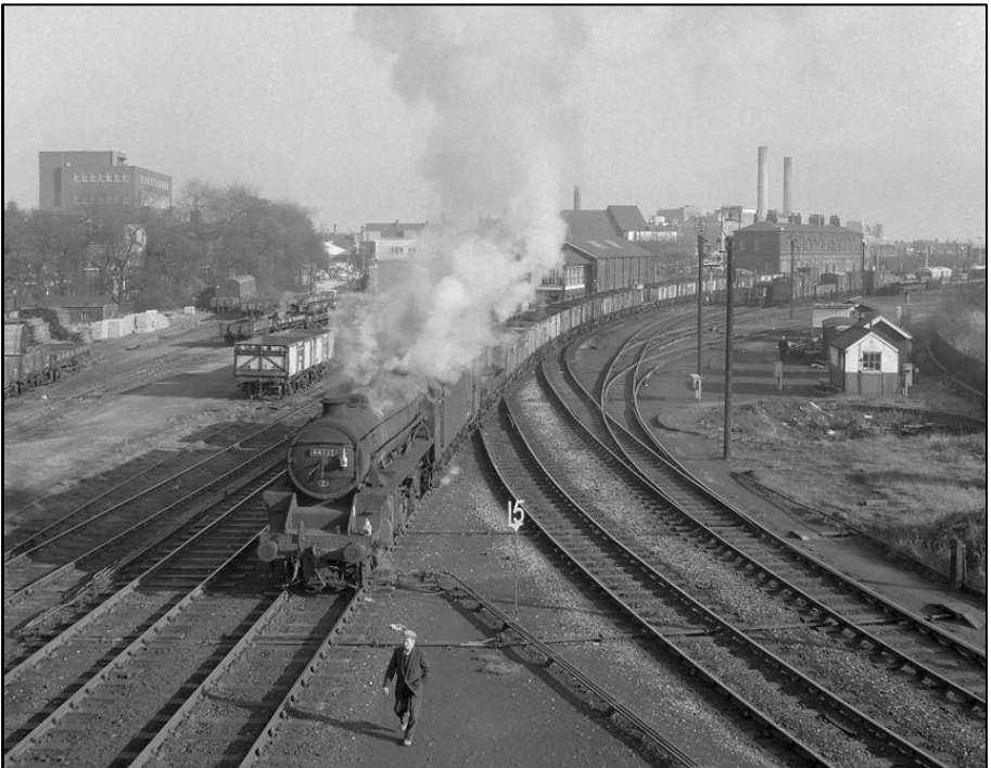
Looking east at Arpley Junction in March 1965. A westbound coal train is seen passing over the junction which was the point at which the W&S and the SHC&RC lines met end on. The line curving to the right provided a connection to the BJR line to Chester. Warrington Arpley station can be seen in the distance. Photo by Eddie Bellas
