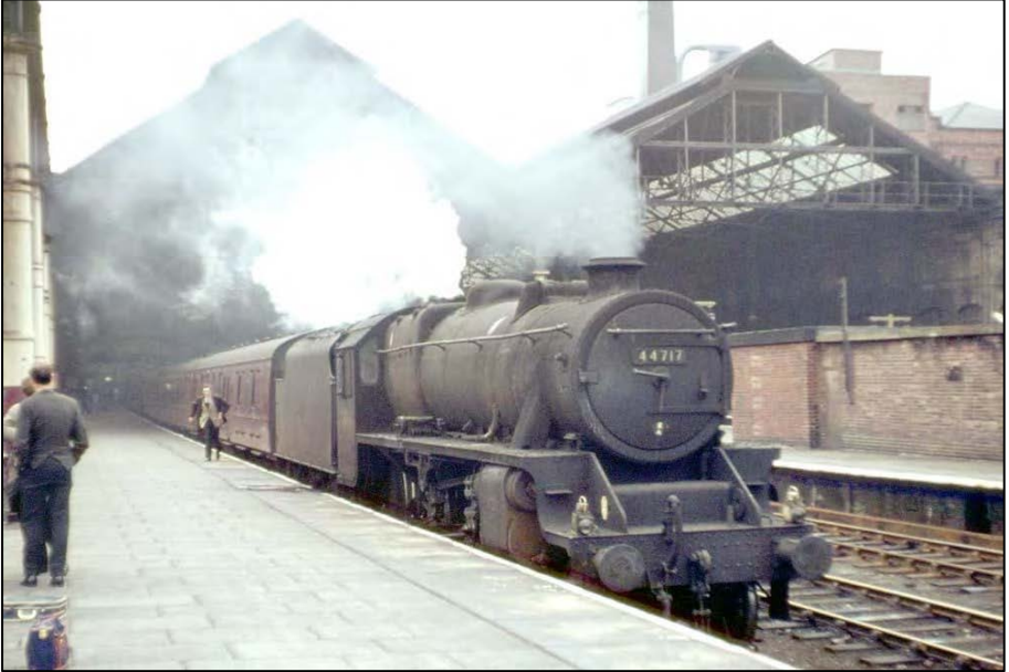
A Glasgow Central service is seen at Liverpool Exchange in 1967. At the head of the train is 4-6-0 5MT locomotive (Black 5) number 44717. Photo by Bevan Price
