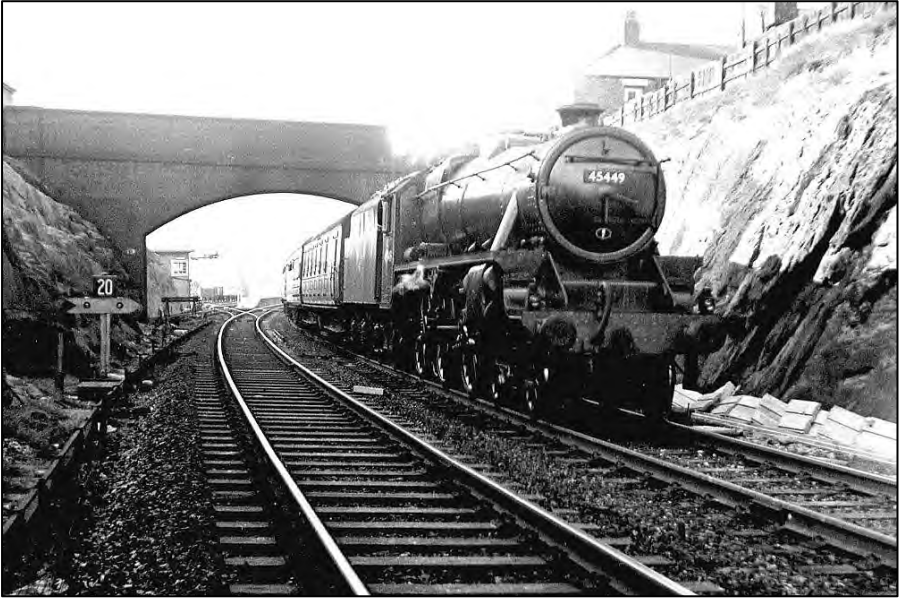
Looking north towards Runcorn station in 1959. Ex-LMS 4-6-0 5MT (Black 5) locomotive is seen on a Liverpool Lime Street to Birmingham New Street service. Photo by Roy Gough
