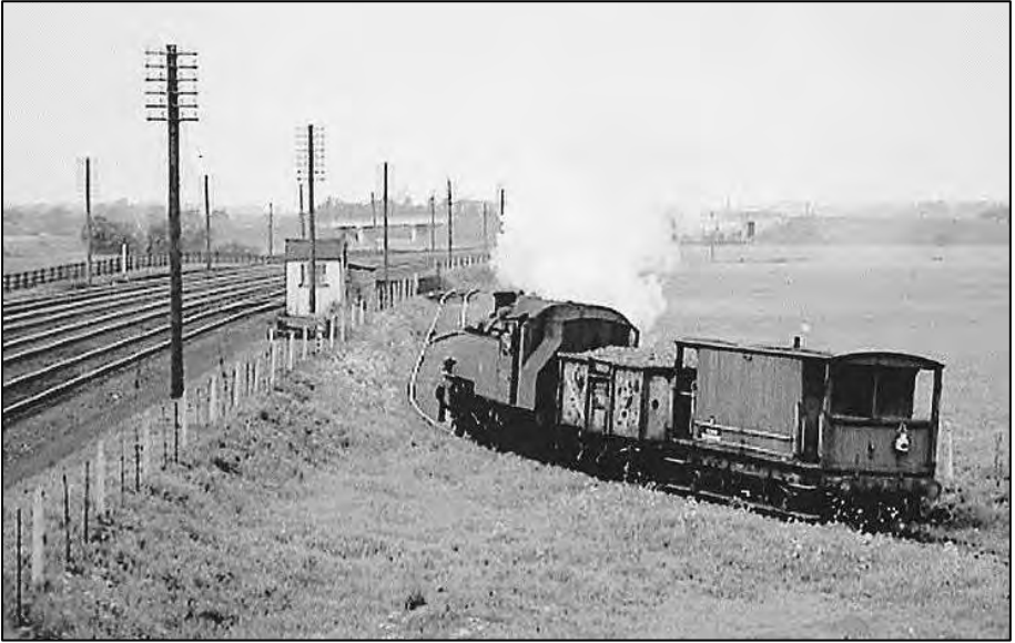
A short train consisting of one 16 ton mineral wagon and a brake van is seen on the Winwick hospital branch in the early 1960s. Providing motive power for the train is ex-LMS 2-6-2 2MT locomotive number 41212 of Sutton Oak shed. Photo by Gerry Drought
