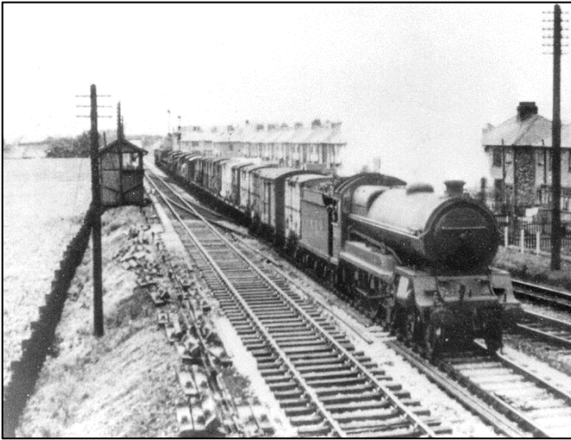
Left: Padgate Junction looking east in the 1930s. Passing onto the avoiding line is a down direction mixed good trains. At its head is ex-GCR B7 class locomotive number 5037.
