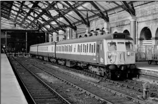
Left: A class 304 EMU at Liverpool Lime Street in December 1989. These units entered service from 1960, and were built specifically for the Liverpool, Manchester and Crewe electrification project. Photo by Doug Birmingham
