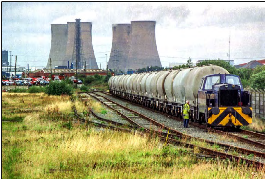
In this view from April 1997 cement wagons have been positioned onto the sidings by the Blue Circle company's own locomotive. This locomotive moved the wagons between the Blue Circle depot and the sidings where main line locomotives would take over. Photo by Terry Callaghan
