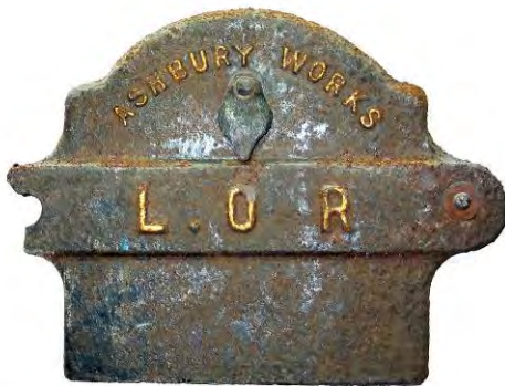
An axle box from one of the LOR 3-car EMUs. It was found by Nigel Wills-Browne and was displayed within the garage for visitors to see. Photo by Tony Foster
