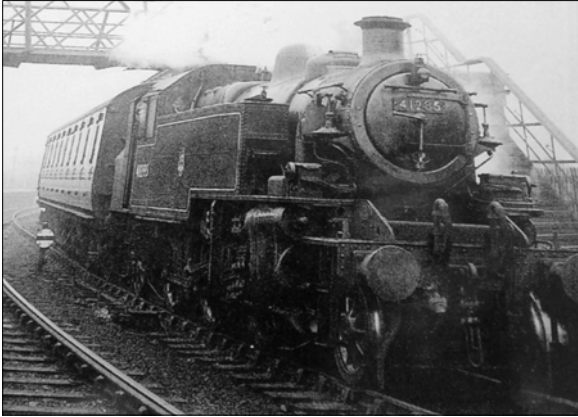
'Push-and-pull' service with Ivatt 2-6-2T No.41285 standing at Earlestown. Note the vacuum valves fitted to the sides of the smokebox.
