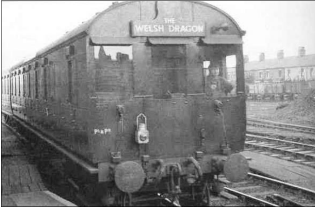
Depicted is a former LMS driving brake second carriage, part of a two coach push-pull set as used on certain local services.
