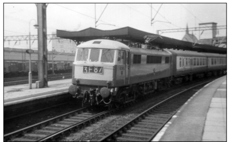
Class AL6 25kv A/c electric locomotive No.E3164 with an express from Lime Street to London Euston. Dated 18 May 1968.
